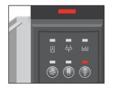
**Precondition**: the Maintenance indicator and the Filter indicator  $\bigcirc$  are illuminated.
